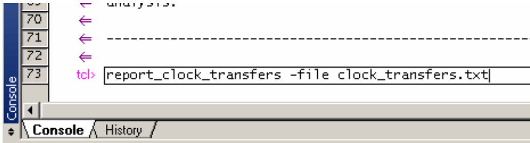
Figure 2–5. Command of Report Clock Transfers for the TimeQuest Timing Analyzer
