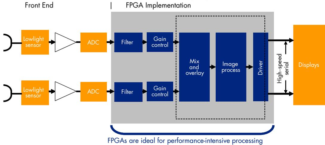
To implement the back-end processing in an FPGA, the designer must create:
