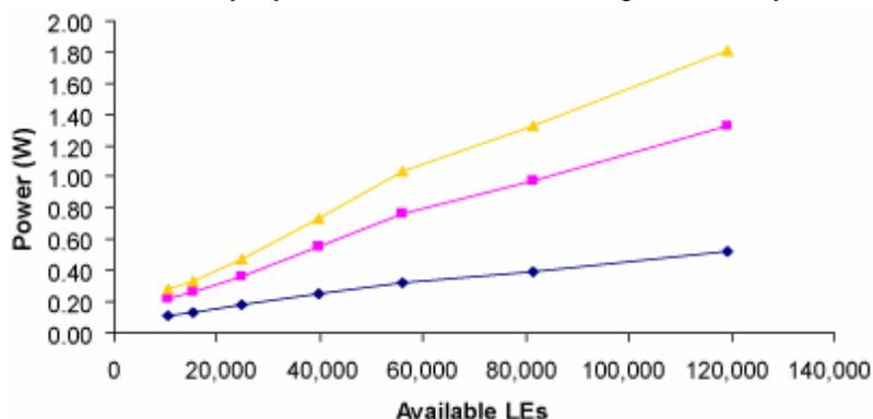
Figure 2 graphs the core static power consumption for various low-cost FPGAs.
