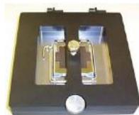
4. The jig is inverted, and paste is applied over the apertures.
