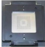
2. The part is hand placed with balls resting in stencil apertures.
