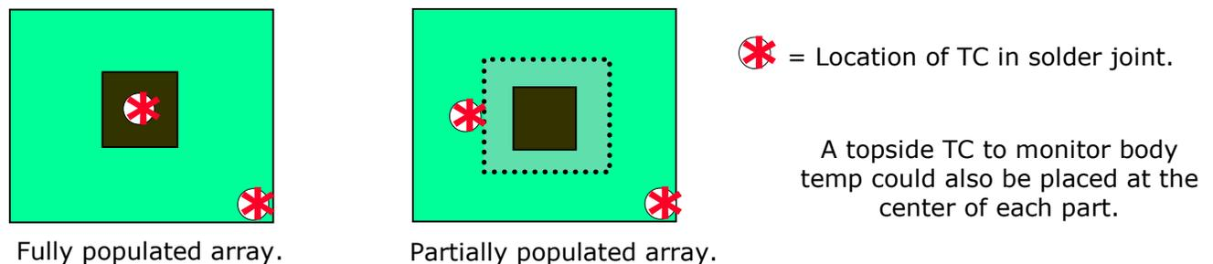
Here is a method for placing TC's to measure SMT joint temperatures:
