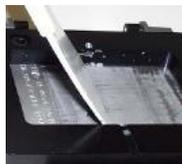
6. The jig is inverted once more, the clamping frame is opened, and the part is removed by the rework machine's vacuum pick for placement onto the board.
