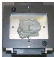
5. A mini squeegee prints paste onto the balls, and removes excess paste.
