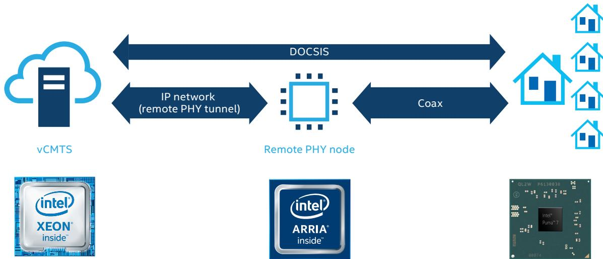
Figure 2. Distributed access architecture with programmable node
