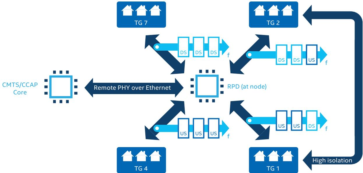
Figure 1. Full duplex communication in an N+0 node
